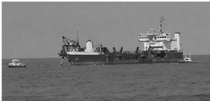
Hopper dredge Liberty Island pumping sand onto John U. Lloyd Beach State Park
